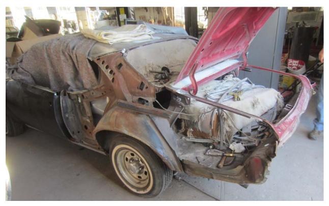
the doors needed rebuilding at the bottoms and the corners as well as new sheetmetal "skins", the front fenders contained hundreds of rust pin-holes that had been puttied over and painted, there was a 3" diameter hole in the roof near the driver's A-pillar – also puttied and painted. It
